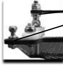
Bump Steer Spacing: 3mm
